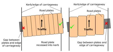
can be staggered and extended on only one side of the carriageway. The full width of openings should be plated to avoid TfL's Lane Rental charges.
