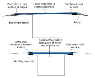
Large steel plates are less likely to follow the road profile than small plates when there is a camber. Bedding material should be used to support the edges, and to prevent rocking and local flexure. Ramps should be formed at edges to smooth vertical height changes greater than 6 mm (see *Traffic Advisory Leaflet 07/96*), taking into account all road users.
